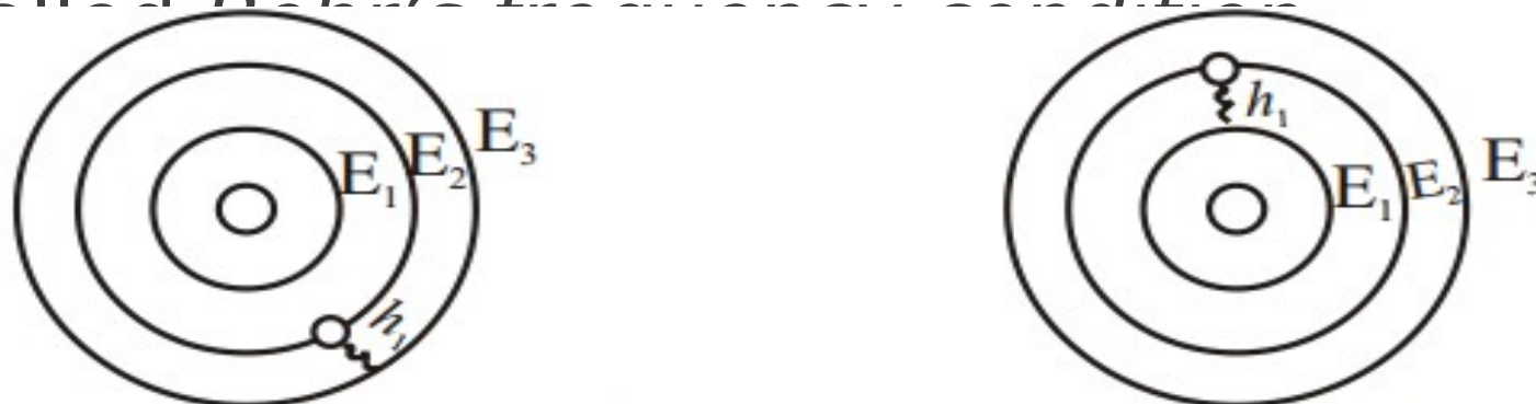
Fig. 3.11 : Absorption and emission of photon causes the electron to change its energy level.
