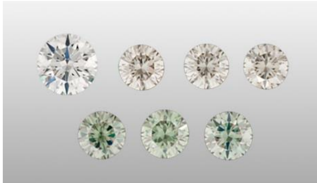
Natural diamond (left), and (inner left to right), laboratory grown moissanite in the near colorless to greenish range
