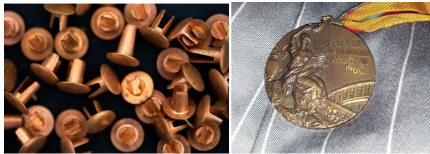
Figure 3 Brass (alloy of Cu and Zn) (left) and bronze (alloy of Cu and Sn) (right).
