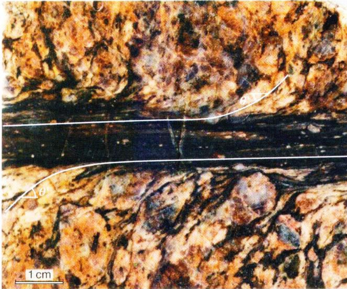
Figure 15.10 A shear zone in the Diana Syenite in Harrisville, New York State, showing profound strain increase toward the central ultramylonitic part of the zone. This is expressed by the change in orientation of the foliation and a marked decrease in grain size in the zone. Photo: Graham B. Baird.
