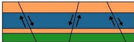
2. Layers are cut by normal faults
