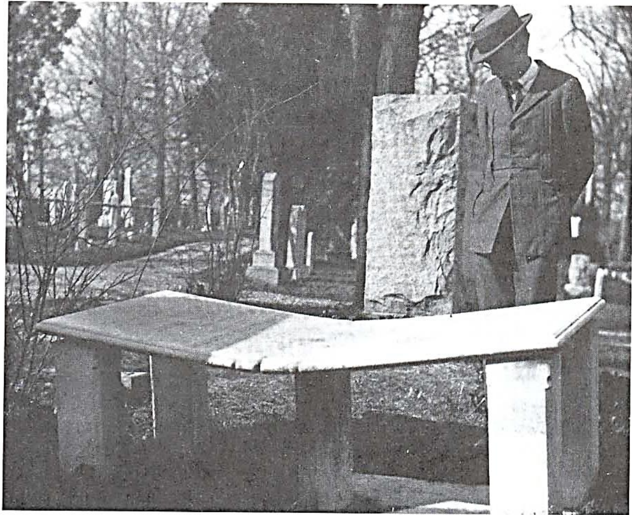
Figure 3.46. Marble bench bent downward by its own weight and that of the occasional occupant. The marble bench is located in cemetery north of Soldier's Home, Washington, D.C. (Photograph taken in 1925 by W.T. Lee. Courtesy of United States Geological Survey)
