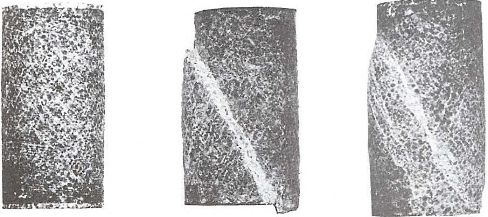
Figure 3.34: Faulted specimens of limestone. (Reprinted by permission. "Some Information Squeezed Out of Rocks". By F.A. Donath. American Scientist. 58, Fig. 7, pp. 54-72 (1970b))
