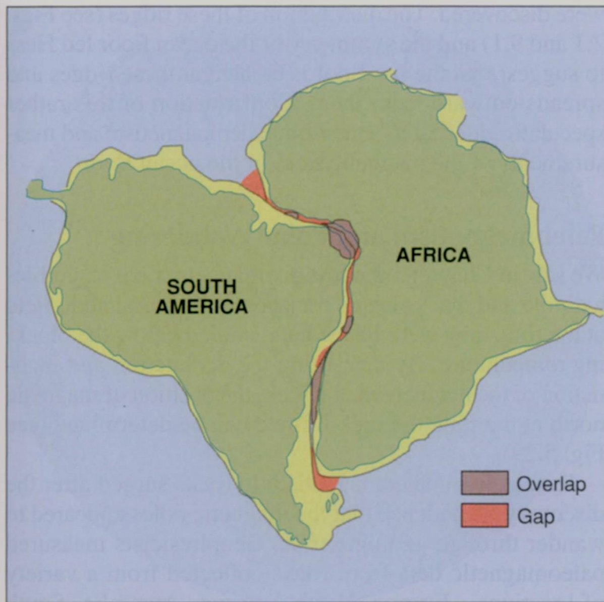
■ FIGURE 7.4 Bullard's fit of South America and Africa. The outlines correspond to the 914-m bathymetric contour. Light red shaded areas represent gaps and gray shaded areas represent overlaps in the fit.
