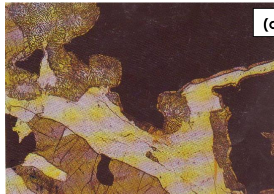
Fig. 18 (c1) Symplectite of iron ore and orthopyroxene; (c2) Fayalite-quartz symplectite
