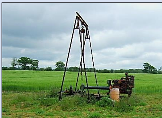
Diesel groundwater pump in use today, England
