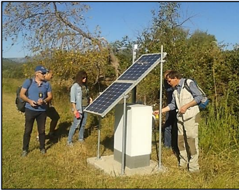
Recording equipment for one of an array of seismometers that is sited in a hole nearby, Gulf of Corinth, Greece
