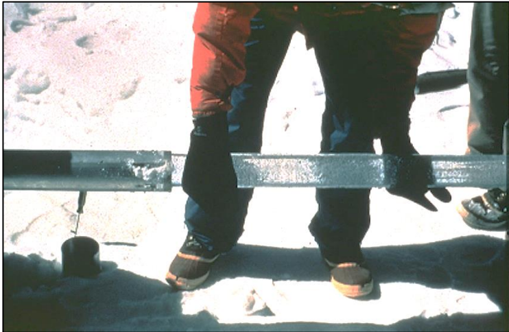
Figure 4.58. Extracting an ice core from a core tube taken from an ice borehole
