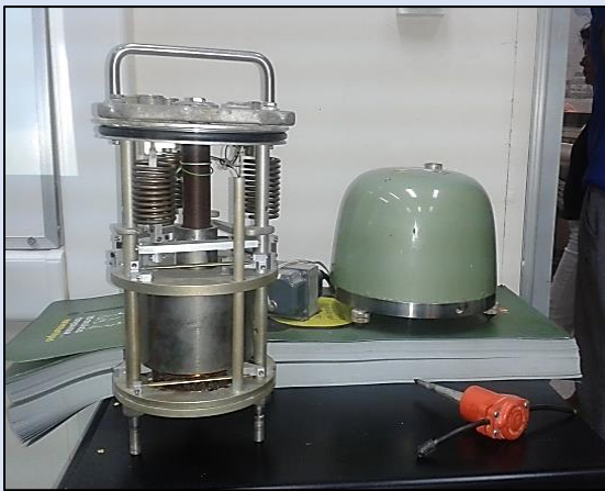
Two seismometers, older one on the left, more modern one on the right, Patras Seismological Laboratory, Greece
