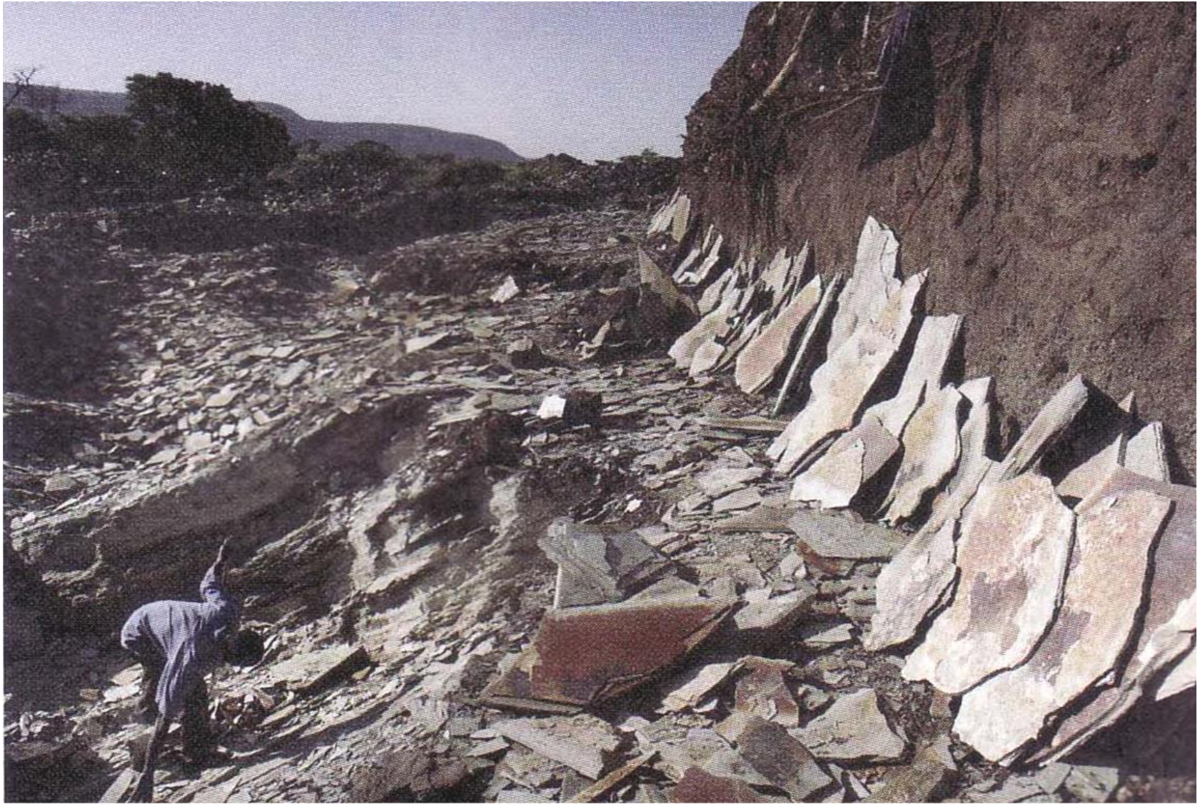
Fig. 8.11. Excellent slaty cleavage is exhibited by the rock in this slate quarry in Tanzania. Because slate breaks into flat slabs, it has many uses (Photo by Randy Olson/NGS image Collection).
