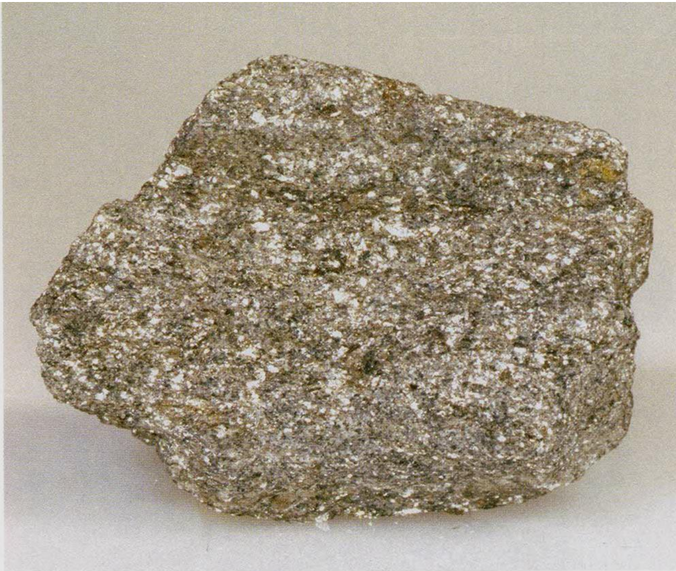
▲ FIGURE 8.15 Mica schist. This sample of schist is composed mostly of muscovite and biotite. (Photo by E. J. Tarbuck)
