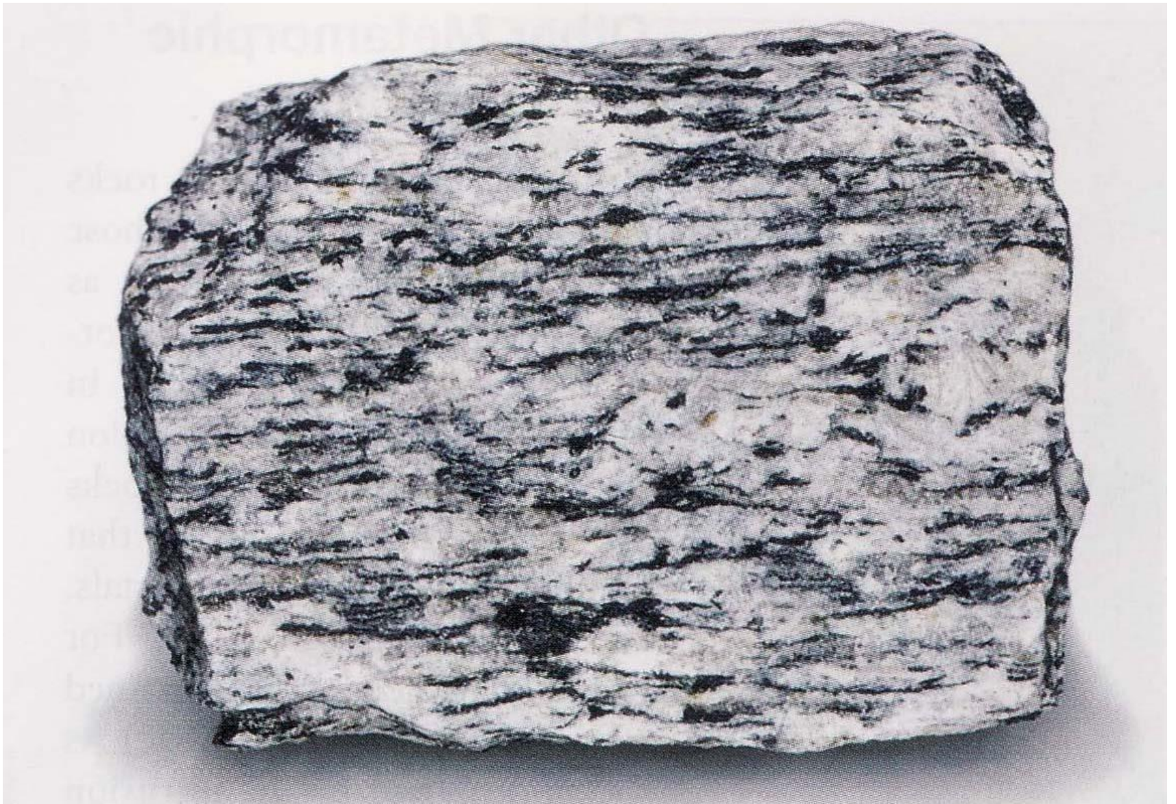
▲ FIGURE 8.10 This rock displays a gneissic texture. Notice that the dark biotite flakes and light silicate minerals are segregated, giving the rock a banded or layered appearance. (Photo by E. J. Tarbuck)
