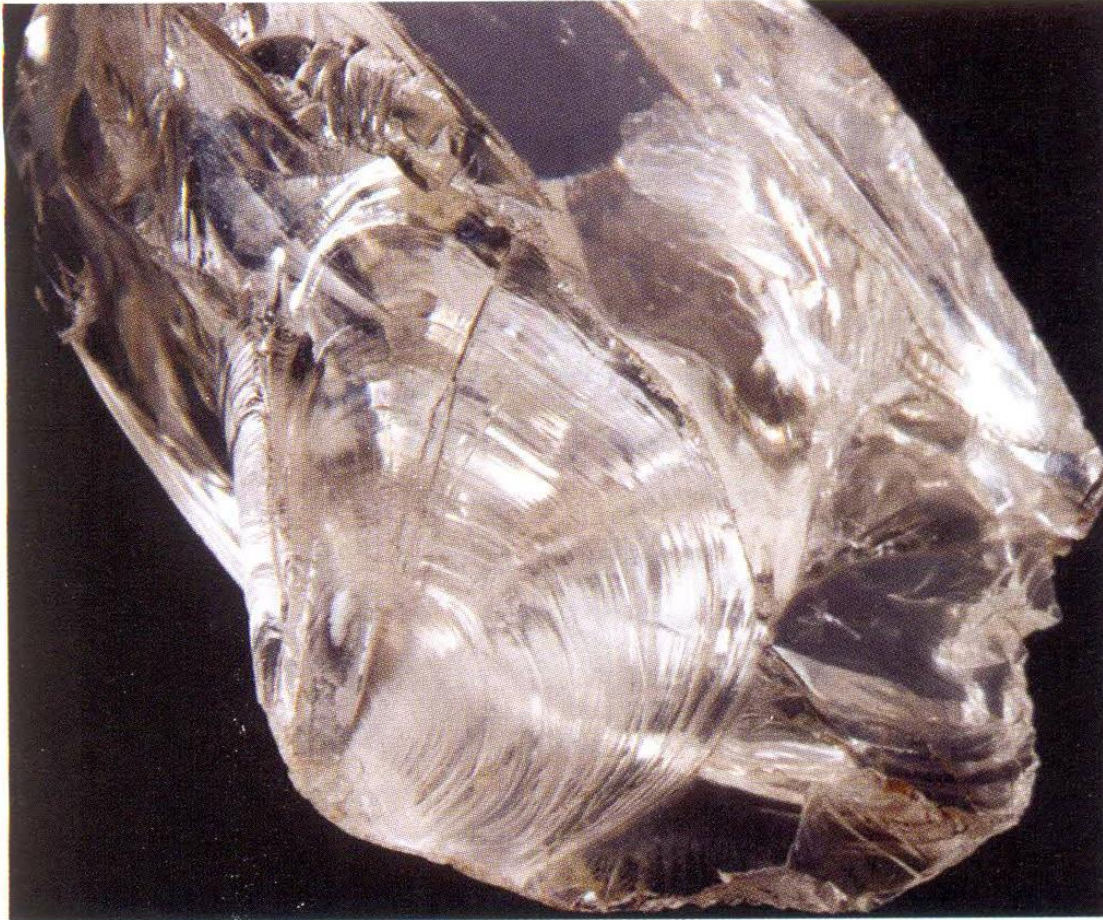
Figure 3.18 Conchoidal fracture as seen in a specimen of clear quartz.
