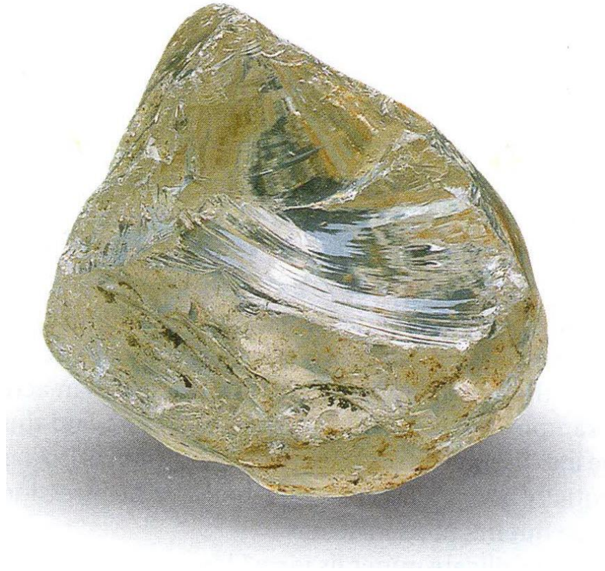
FIGURE 2.18 Conchoidal fracture. The smooth, curved surfaces result when minerals break in a glasslike manner. (Photo courtesy of E. J. Tarbuck)
