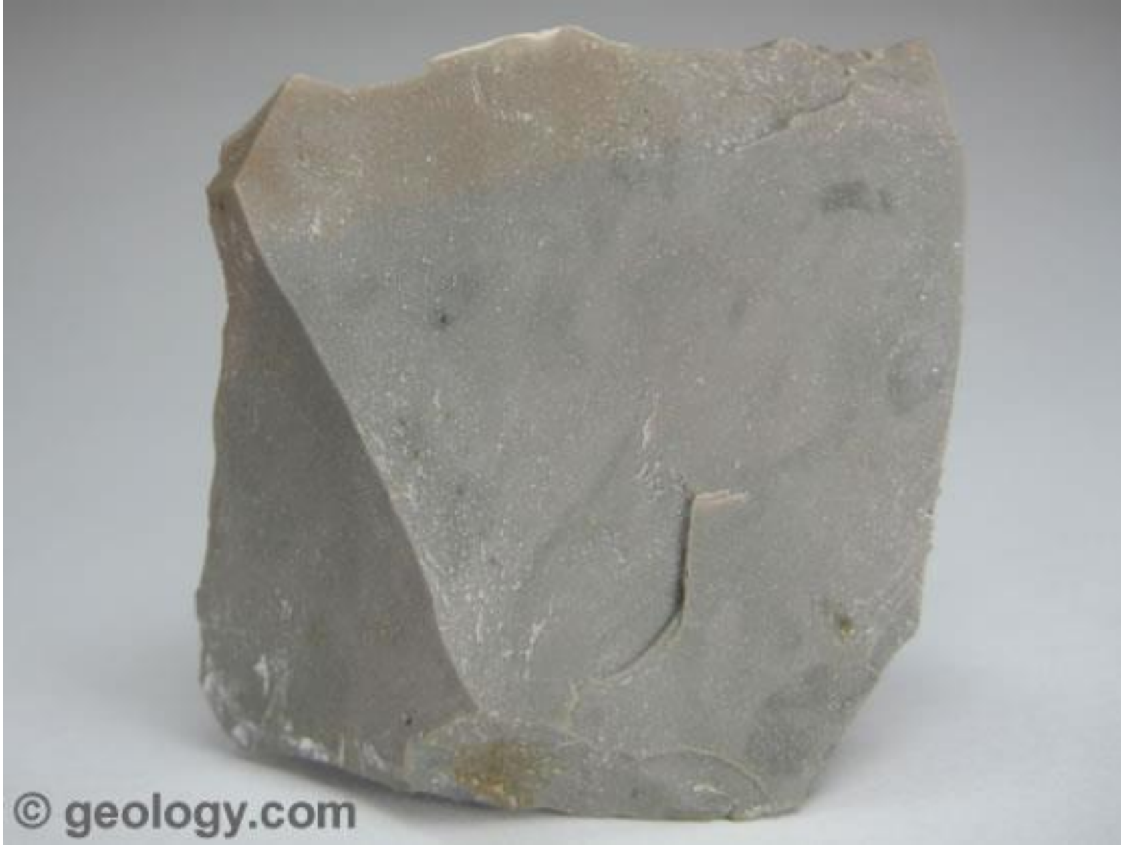
Chert: This specimen of chert is about two inches (five centimeters) across. It displays conchoidal fracture and has broken to produce sharp edges.
