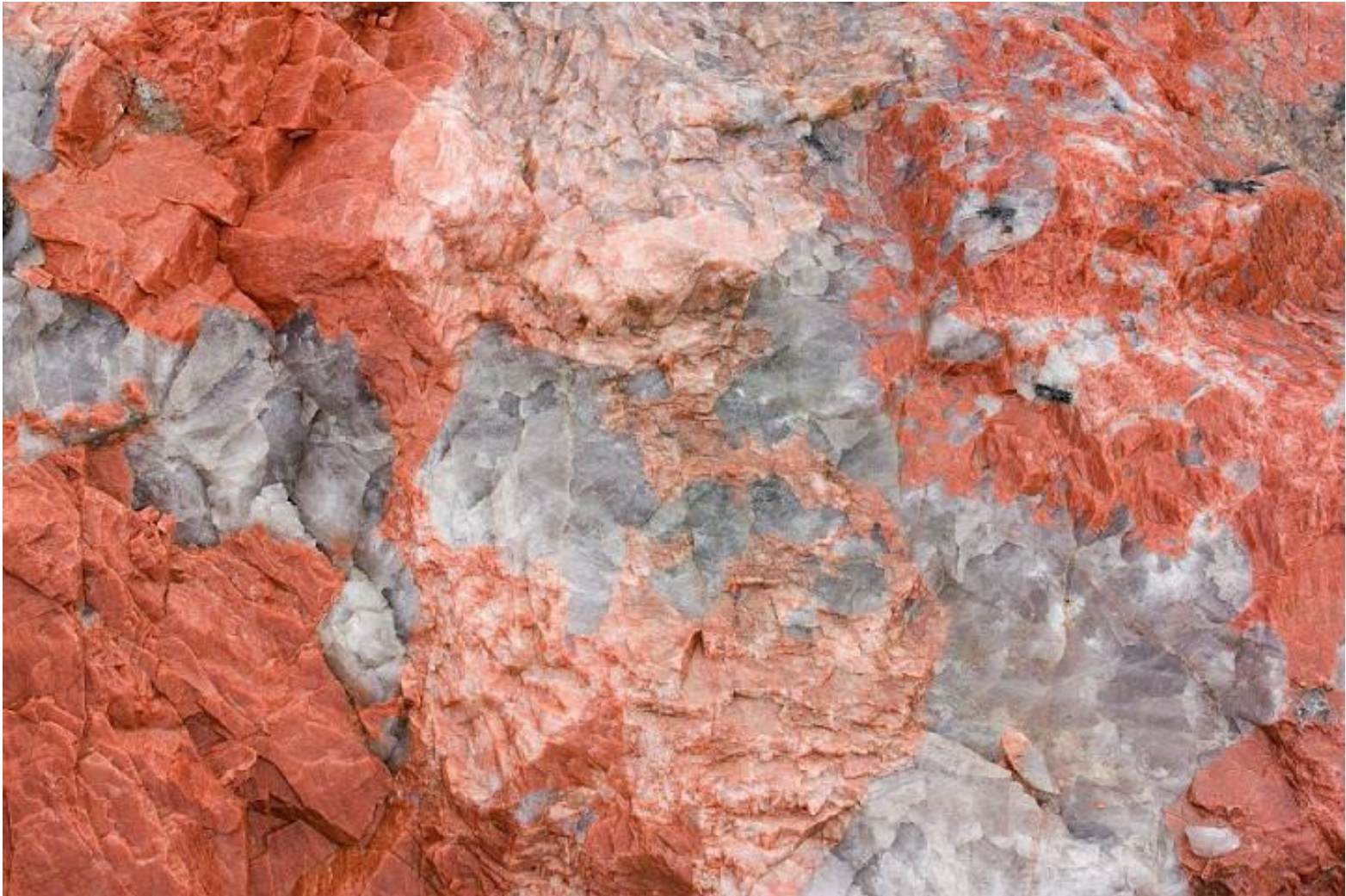
Pegmatite is a very coarse-grained igneous rock. Simple pegmatites are composed of large crystals of ordinary minerals. Here is a sample of alkali feldspar granite pegmatite from Northern Norway which is composed of alkali feldspar (pink), quartz (gray) and biotite (black). Width of view 50 cm.
