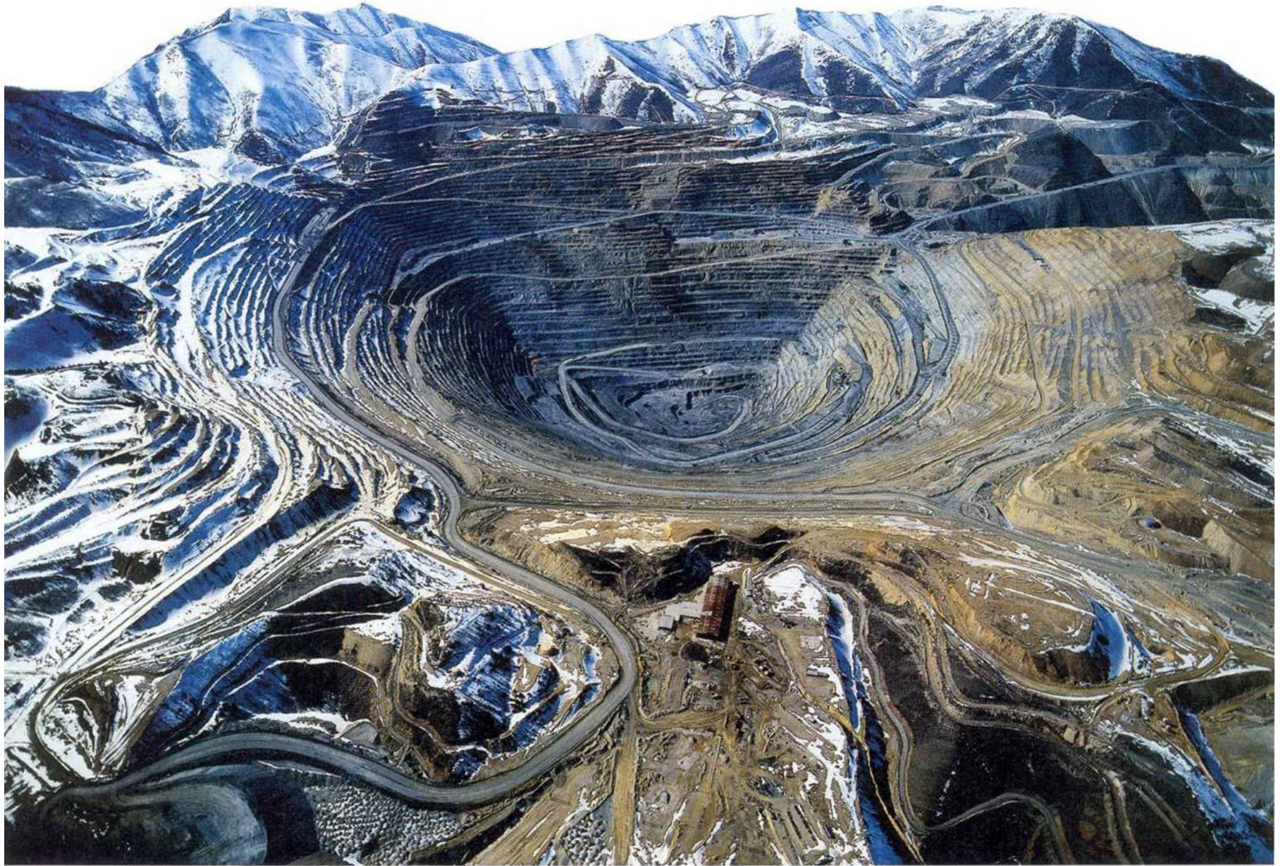
FIGURE 2.27 Aerial view of Bingham Canyon copper mine near Salt Lake City, Utah. Although the amount of copper in the rock is less than 1 percent, the huge volume of material removed and processed each day (about 200,000 tons) yields enough metal to be profitable. (Photo by Michael Collier)
