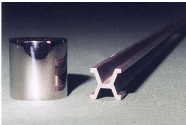
Figure 1: The International Prototype Kilogram (IPK) and Standard metre held at BIPM in Paris, France. The standard metre is made to be exactly the length that light could travel in 1/299\,792\,458 of a second.
