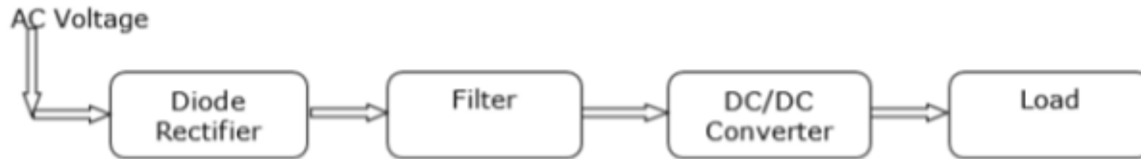
Fig. 2.2 - DC Power Supply
