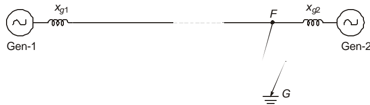
Fig. 8.11 Line-to-ground fault on a system with multiple generation to illustrate initiation of travelling waves.
