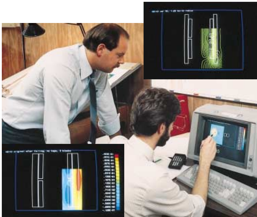
FIGURE 1–2 A transformer designer using a 3-D electromagnetic analysis program to check the design and operation of a power transformer. Upper inset: Magnetic field pattern. (Courtesy Carte International Inc.)
