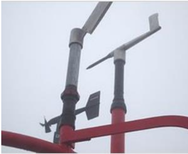
Weather instruments at Mount Washington Observatory . Pitot tube static anemometer is on the right.
