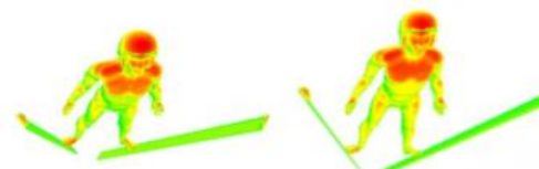
Fig. 2a. Distribution of aerodynamic drag coefficient (FLA of 20°)
