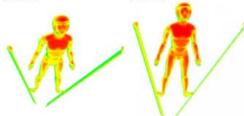
Fig. 2c. Distribution of aerodynamic drag coefficient (FLA of 40°)
