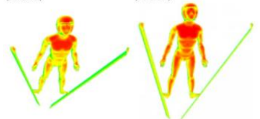
Fig. 2c. Distribution of aerodynamic drag coefficient (FLA of 40°)
