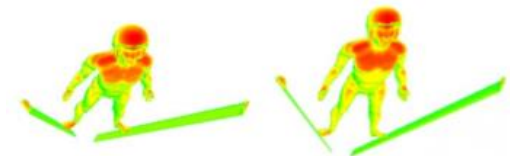
Fig. 2a. Distribution of aerodynamic drag coefficient (FLA of 20°)
