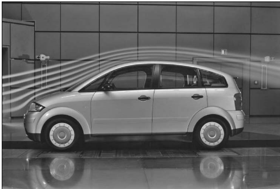
Fig. 2.4 Streaklines over an automobile in a wind tunnel. (Courtesy Audi AG.)
