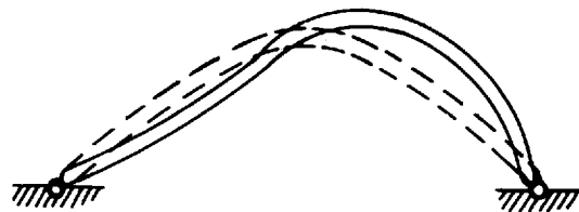
Arch buckling (in plane)
