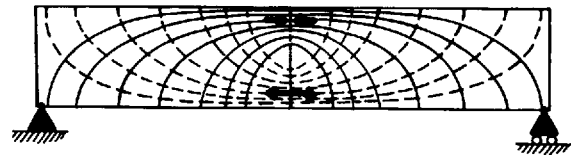
Principal stress trajectories in a simply supported beam
