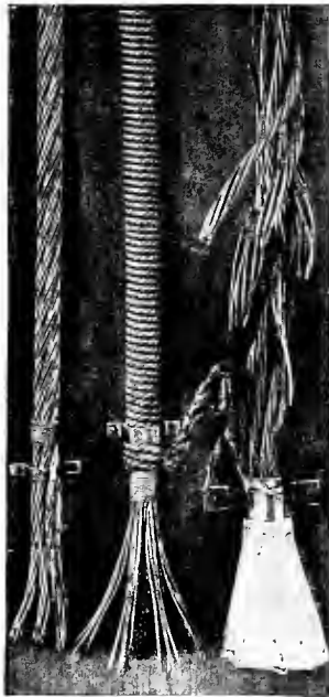
FIG. 244.—Method of capping wire ropes.
