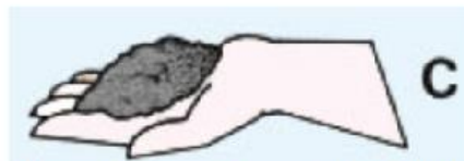
If the soil fall apart, its poor with too much sand
