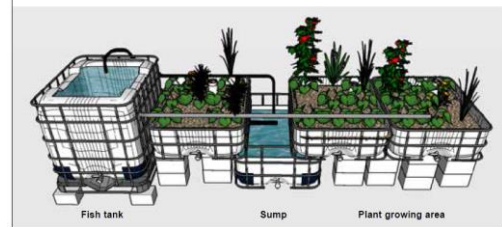
Illustration of a small media bed unit
