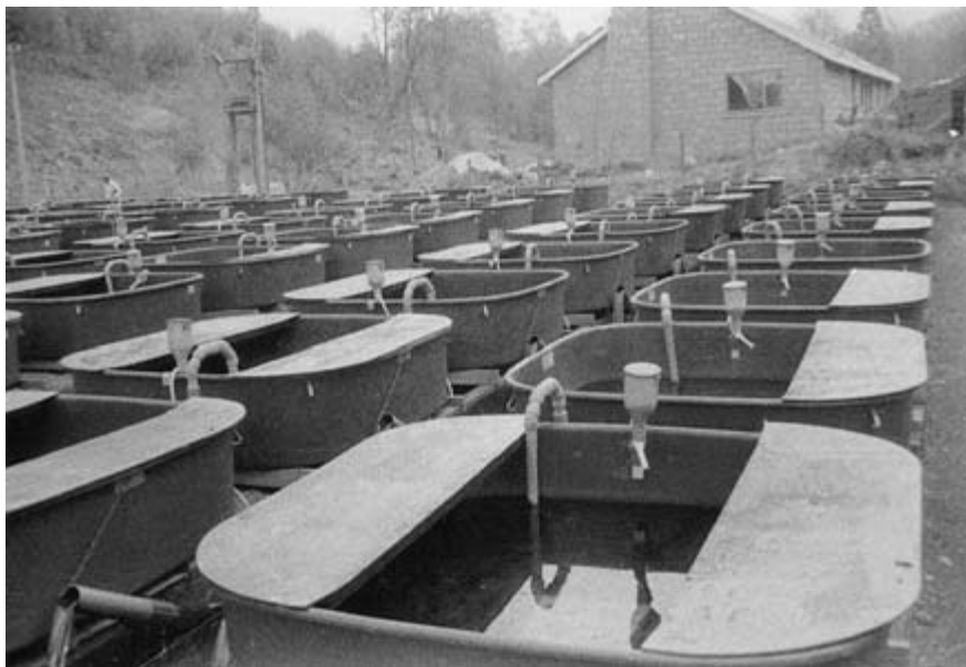
Fig. 6.18 An outdoor tank farm. Tanks are made of fibreglass.
