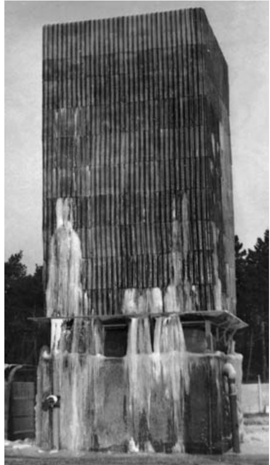
Fig. 6.35 Deepwell water being aerated through a tower for hatchery use in Poland. (Photograph: J. Walugo.)
