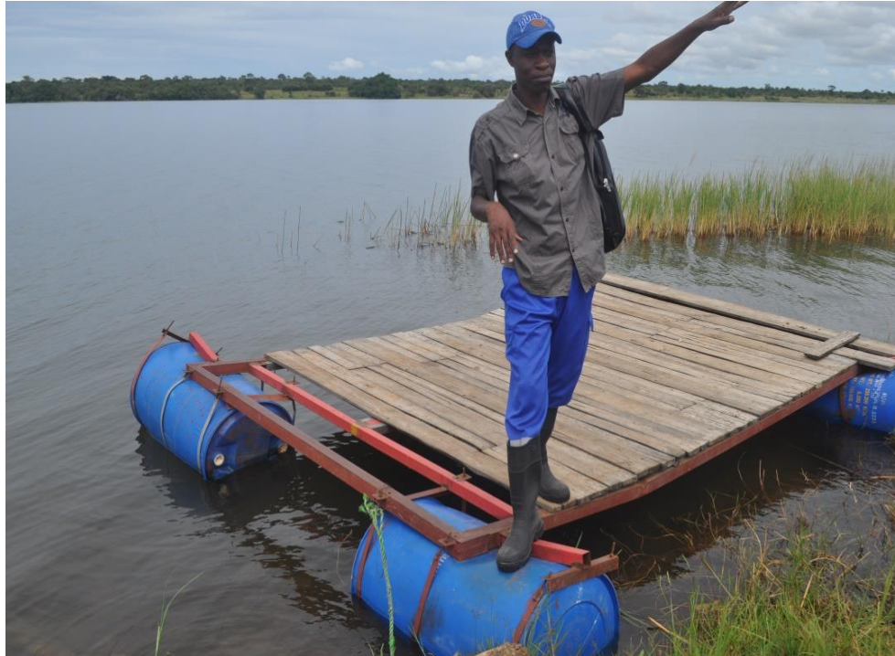
Raft for transport and management of cages
