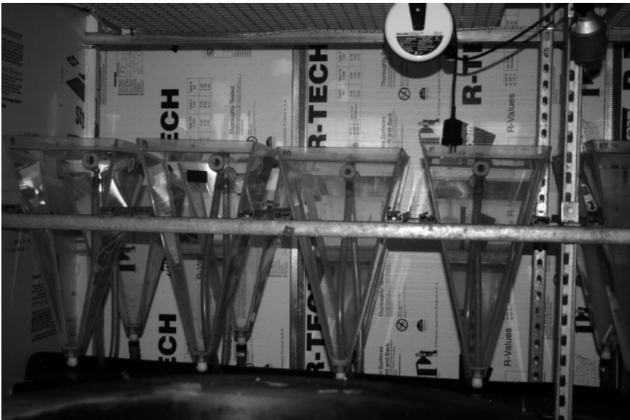
Fig. 1.2. Plexiglass containers used to hatch marine fish eggs in a research laboratory.
