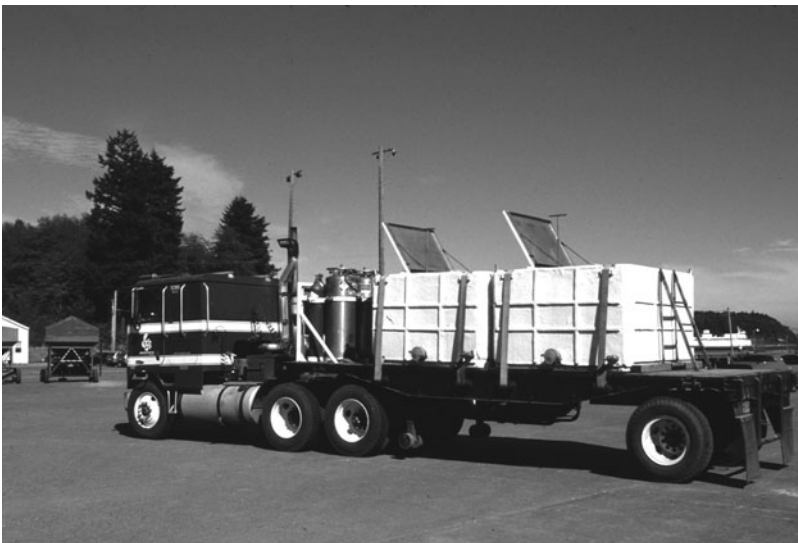
Fig. 8.3. A truck with large tanks that can be used for hauling fish or shellfish on ice to the processor.
