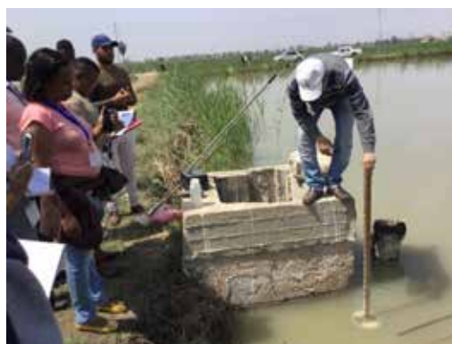
Figure 54: How to take Secchi Readings
