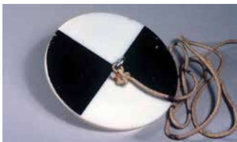
Figure 53. The Secchi Disc
