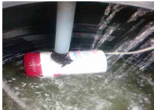
(b) Submersible Pumps. Normally placed inside unit with filtered water
