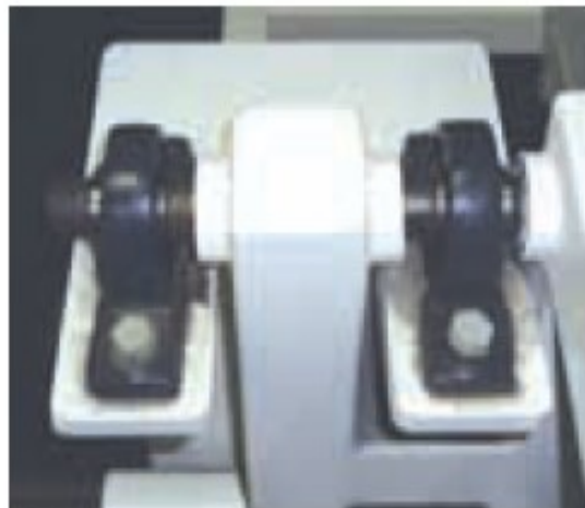
The journal bearings support the ends of the shaft. (5) (© Russell C. Hibbeler)
