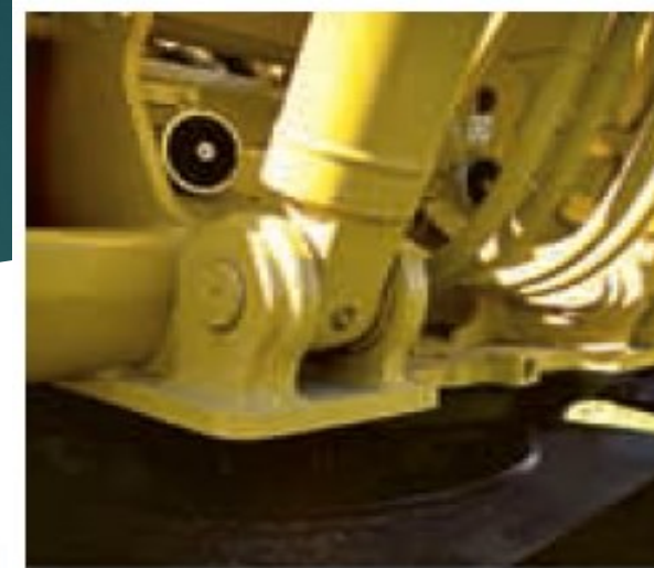
This pin is used to support the end of the strut used on a tractor. (8) (© Russell C. Hibbeler)
