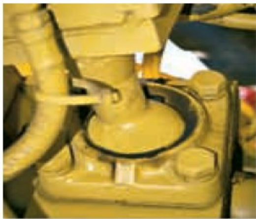
This ball-and-socket joint provides a connection for the housing of an earth grader to its frame. (4) (© Russell C Hibbeler)
