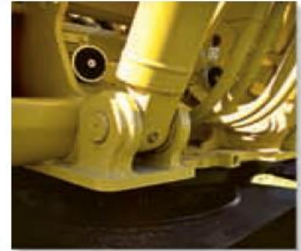
This pin is used to support the end of the strut used on a tractor. (8) (© Russell C. Hibbeler)
